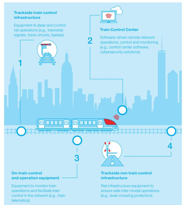
The train control and signaling segment provides all elements to safely operate and monitor a rail network and to utilize the infrastructure capacity efficiently. The signaling product space is highly complex and includes various physical assets along the tracks, within trains, and in remote control centers - all of which need to be inter-connected. While today, the high variety of an OEM's product
