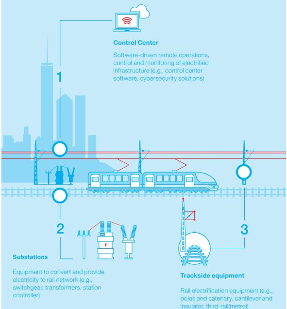
The rail electrification segment is comprised of all elements to convert and deliver electric energy directly to trains. Substations convert energy from national networks into the right frequency and voltage used in rail operations. For energy transmission along the track, two main systems dominate – catenary in mainline operations and third-rail in metro systems. Control centers
